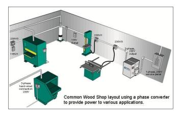
When confronted with this dilemma, a shop owner can choose to 1) purchase only single-phase machinery 2) Convert 3-phase machines to operate on 1-phase, or 3) Use a phase converter to operate the 3-phase machines from a 1-phase supply.
